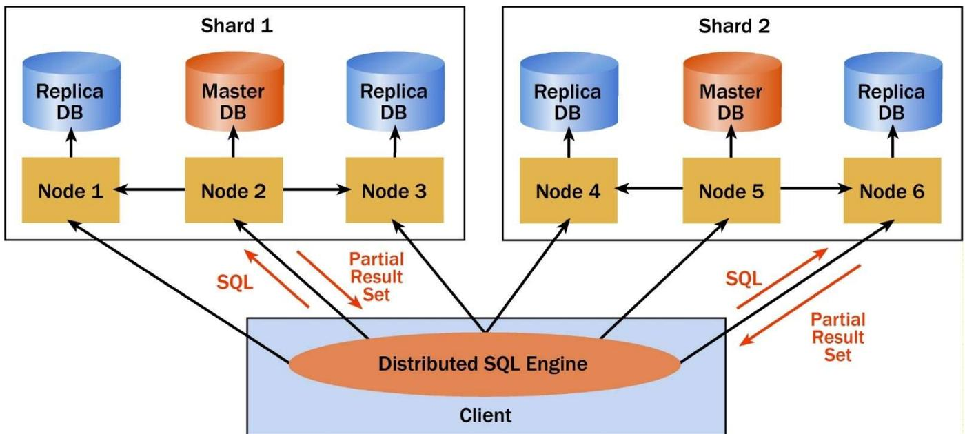
**Sharding, with distributed query processing, leverages the processing power, memory and bandwidth of multiple hardware nodes. Each database shard can have one or more backup (replica) copies to ensure continuous availability.**
