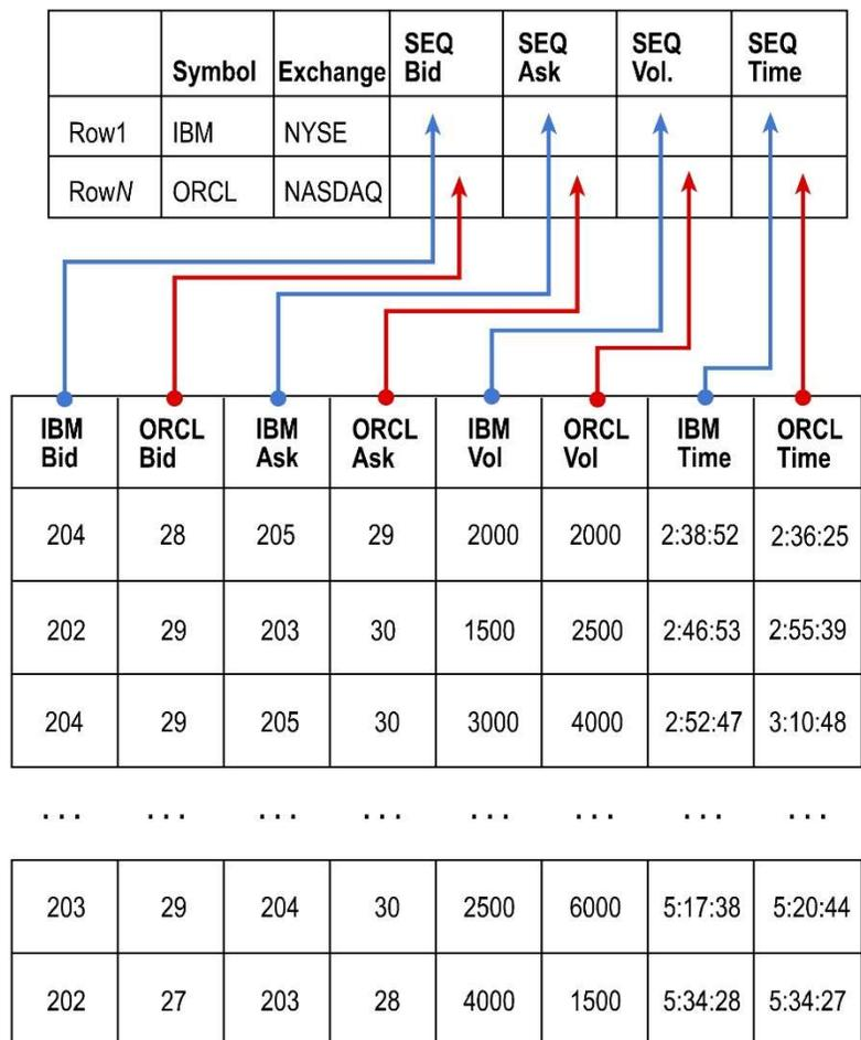
**Traditional DBMSs bring rows of data into CPU cache for processing. But time series data – such as IoT, ticks, trades and quotes – are better handled by a column-based layout that maximizes efficiency in fetching needed information.**
